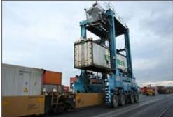
Figure 2: a straddle carrier at work
