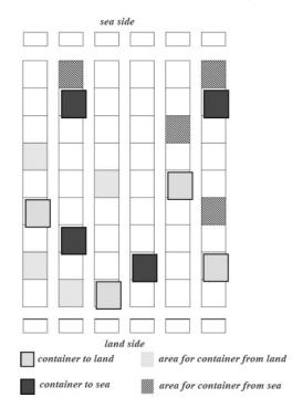
Figure 3: schematic representation of a stack block
